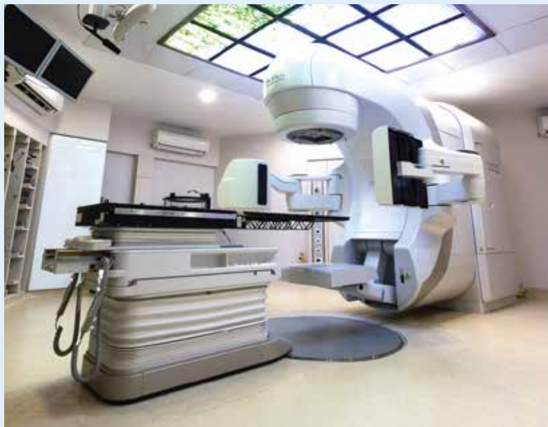
▶ Advanced Linear Accelerator with prone breast radiation therapy
